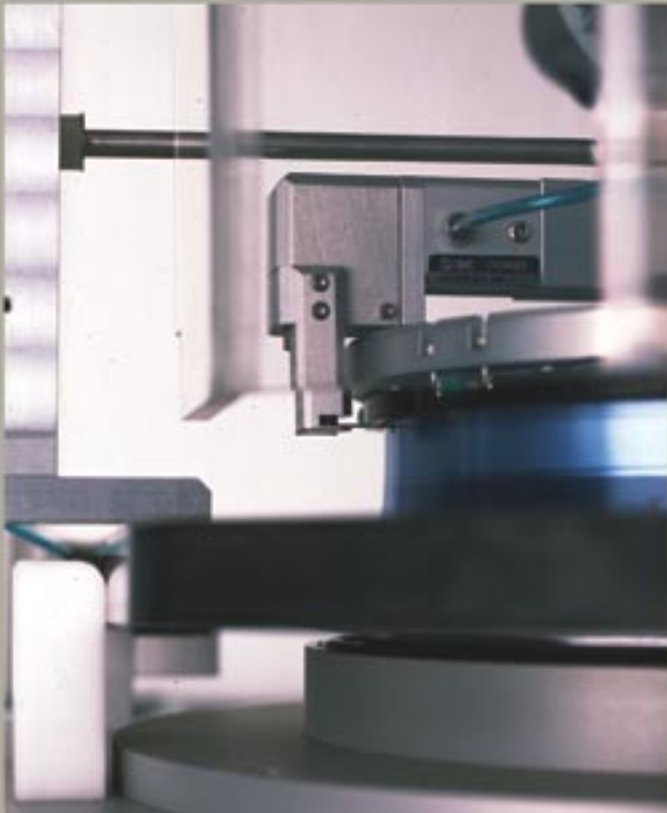
Close-up of optional motorized cutter and plexi cover.
