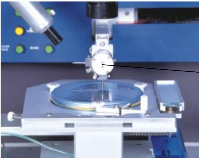
Detail of Bond Head Assembly with Preform Pickup Tool
