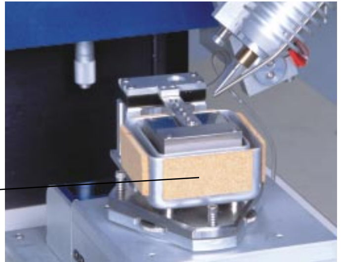
Motorized Workstage with Pneumatic Package Holder
